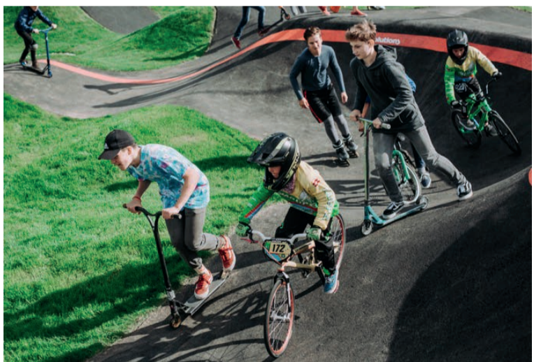
Safety Lines and Landscaping Painted lines partly follow edges of the pump track to give a visual indication of track layout and guide riders around. The embankments and interior areas of the track are to be turfed with an amenity grass to ensure landscape is protected and hardwearing.
