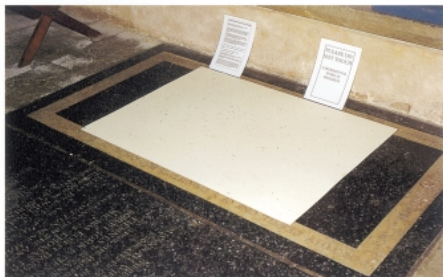
The church at Broughton, Oxfordshire, was used as part of the experimental work in developing a number of ways that parishes could begin to monitor and ameliorate a bat problem. Here one metre square cards were positioned over an area of the chancel floor. These were left in place for a number of months during which time individual droppings and urine droplets were systematically counted. This yielded useful baseline data on the active rate over time of the deposition of bat excreta occurring in this part of the church
